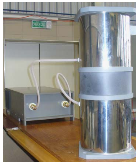
Figure 1. Portable repetitive source of 150MHz frequency
