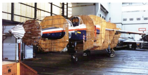
Figure 2. Example of return conductor setup
