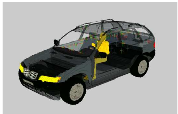
Figure 1: Driver and car meshing obtained with the “Nash” FDTD mesher in the Quercy2 simulation platform
