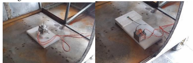
(a) 3D electric field sensor (b) 3D magnetic field sensor Fig. 3. Measurement of transient electromagnetic field
