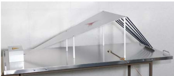
Fig. 1 Picture of the Montena Technology EMP25K-2-23 small NEMP simulator
