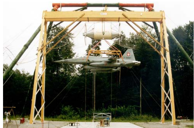
Figure 1. EMP test of Swiss Tiger F-5 in MEMPS facility
