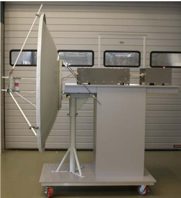
Figure 2. Portable repetitive source of 1GHz frequency with the dish reflector
