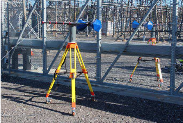
Figure 2: SEMS antennas measuring the SE of a perimeter fence
